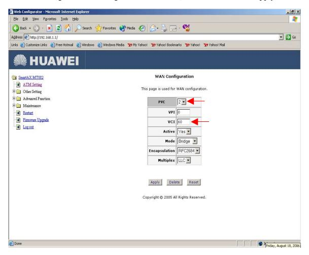
(This is required for router configuration on the first time because router is to be configured on PVC 0 and VPI 0 & VCI 32)
