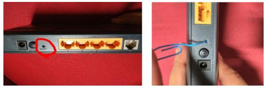
Press the RESET button with pointed object like pin or pen for 5 seconds or till all LEDs on modem go down and modem reboots.
