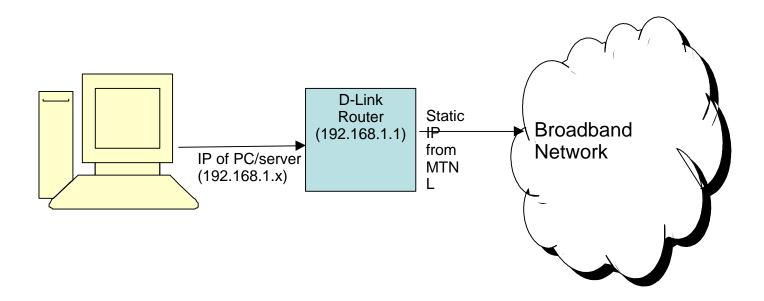
Note: Since NAT enabled in ADSL router Static IP will be allotted on WAN side and private IP 192.168.1.x will be allotted to the machines connected to the router as shown above.
