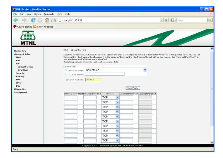
3) Select the application which is to be configured with static ip (webserver, ftp,telnet,vpn etc) from the **Select One** drop down menu
