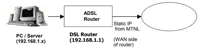
Note: Since NAT enabled in ADSL router Static IP will be allotted on WAN side and private IP 192.168.1.x will be allotted to the machines connected to the router as shown above.
